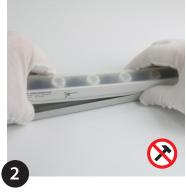
Carefully push-fit MOMO Flex into the linear rail, starting at one end and pushing down with a uniform force working along the full length until seated correctly - This should be done manually without tools that could damage the silicone housing.
