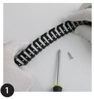
For curved forms the metal linear flex clip can be screw fixed to a compliant surface with compatible screws.
