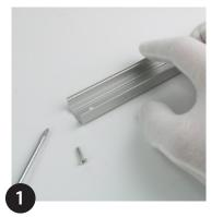
For fixed straight runs, the linear aluminium rail can be used. Screw fix the rail to a suitable flat mounted surface with compatible screws.
